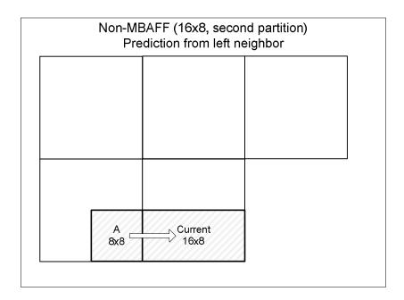
For the rest cases the predicted motion vector is either identical to one of the neighboring motion vectors or it is the median of the three candidates. The derivation of the predicted motion vector (MVP) is illustrated in the following pseudo-code:
