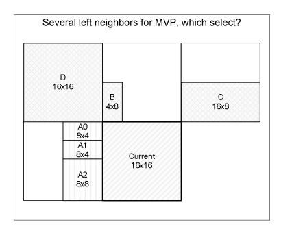
In case of several left neighbors (e.g. in the above figure the current 16x16 block has three left neighboring blocks A0, A1 and A2) the "topmost" rule is applied to select non-ambiguously the block for prediction: from all left neighboring blocks always select topmost (in the above figure the block for prediction is A0).
