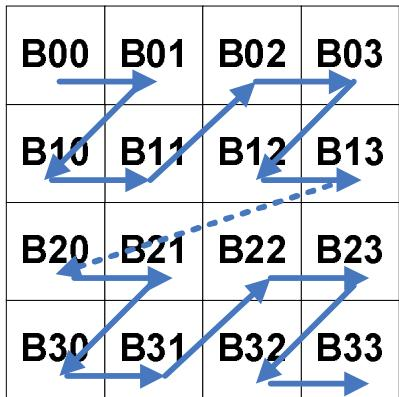
In the above figure  $B_{ij}$  means  $(i,j)$ -th  $4 \times 4$  sub-block, the zig-zag-like line shows the decoding order. We can't process B01 and B10 in parallel since top-right predictors for B10 are taken from the reconstructed samples of B01. However we can process simultaneously blocks B02 and B10. Moreover blocks B03 and B11 can be processed in parallel.
