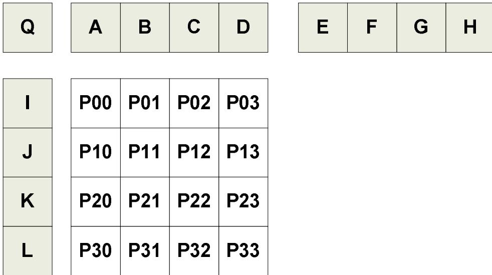
[A,B,C,D] are top samples, [E,F,G,H] – top-right samples, [I,J,K,L] – left samples and Q is top-left sample respectively. The following sub-sections describe how to calculate predictors for all 4x4 luma intra modes (except horizontal and vertical due to triviality).
